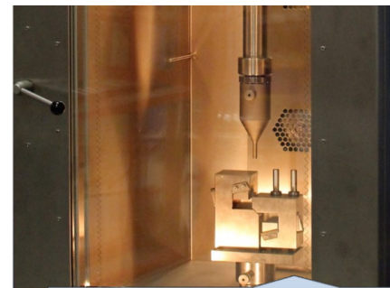
Temperature chambers with a range from - 196 ° C to + 350 ° C.
