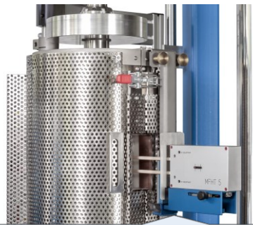
High temperature furnaces up to temperatures of 1600 ° C.
