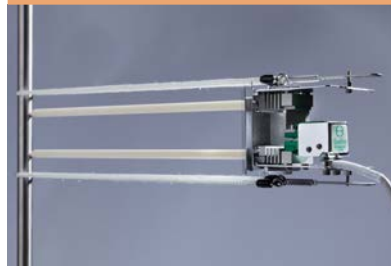
The Model 3448 is self-supporting using reusable ceramic cords
